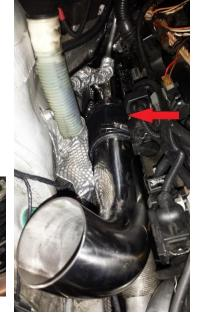
3) PCV System - Cut a short 6 inch piece of 1" silicone hose and connect to the OEM PCV check valve that sits
