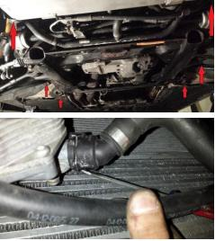
21) Coolant – From underside of engine you will see an aluminum box-like unit attached to the fan. Remove the locking clip from the small plastic fitting on the heater hose connected to it. Make sure you have a drain pan or a bucket with you to catch the coolant. Once drained, remove the T-25 Torx scre holding the aluminum box assembly from the fan. (sorry I do not know what this thing is called and it is driving me nuts)
